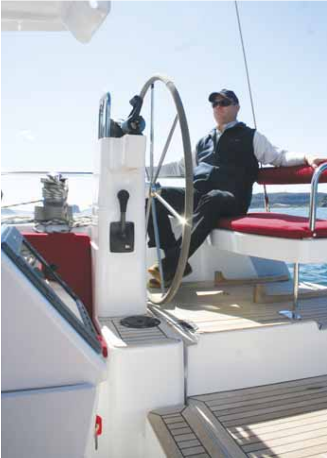
You can't complain about the comfort of the steering stations. Teak chocks beneath seat are for liferaft.
